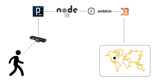
In News Explorer, the XY coordinates and depth information is normalized and sent to a NodeJS web-server via Open Sound Control (OSC) protocol. The NodeJS web-server efficiently transmits this information to a web page using the WebSocket protocol, ensuring a lag-free experience. The web page consists of a world map and a circular cursor, rendered using D3.js JavaScript library. As
